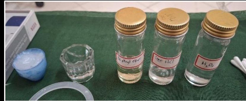
Preparation of McInnes solution using 30% H_2O_2 , 36% HCl and 0.2% Ether
